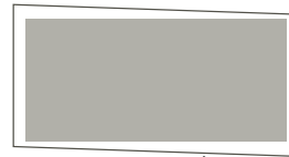
POOR BASE POSITIONING (CORNERS NOT AT RIGHT ANGLES)
